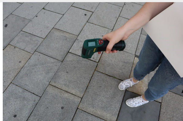
Figure 48 - Measure surface temperatures using infrared thermometer in city center (Author: 3 E PROJEKTI d.o.o.)
