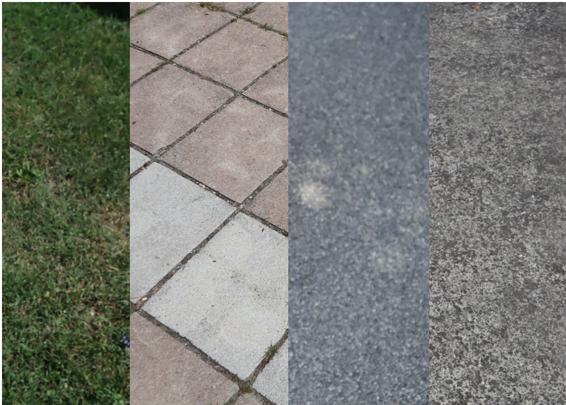
Figure 33 – Materials type (from left to right: grass, concrete pavers, asphalt and concrete ) in study area of flea market (SAJMIŠTE) (author: 3 E PROJEKTI d.o.o.)
